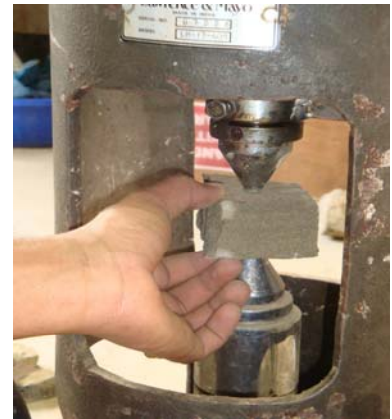
Determination of rock strength (Point Load Test)
