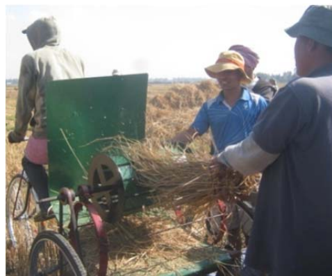
Trial of Harvesting of paddy using paddy thresher in progress
