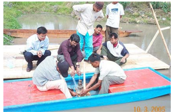
Inclination test of 3m FRP boat
